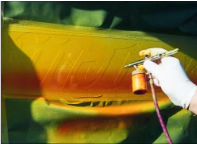
The next color that I airbrush is medium orange. Starting at the bottom, I spray a little more than half way up the letter. Don't bother to clean out the airbrush between colors, they're in the same family.
