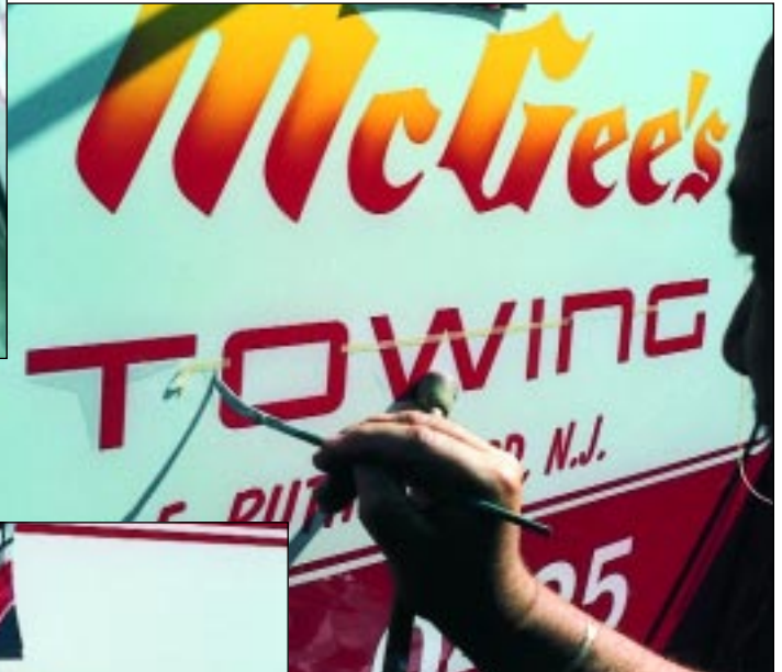
The remainder of the copy is done in high-performance vinyl. (I don't use intermediate or economy vinyl for truck lettering.) Using a #8 brown lettering quill, I paint a light gray shade on the words "TOWING" and "Local & Long Distance". This mix is white, imitation gold and some black. Again I add a couple of drops of hardener and some hi-temp reducer. (Mix your grays a couple of shades lighter than what you'd like it to look like after it dries because it always dries darker.)
