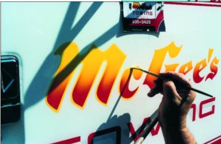
For some extra color and to separate the bold outline, a mix of chrome yellow and a little polar white is applied to the outside of the airbrushed letters. I'm using a cut-down #8 brown lettering quill. (Trim the brush at the ferrule, cutting around the brush next to the ferrule. Never cut the brush at the tip.)
