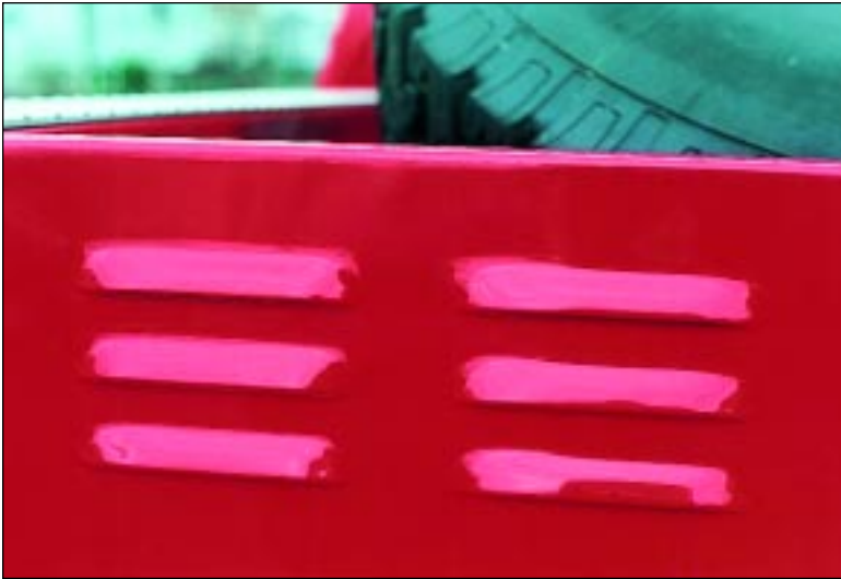
This is one of the reference photos that I used as my model for the louvres. It's the most popular style and measures about 3/4" x 3 1/2" long. There are of course other sizes and styles. (Check out hot rod and truck magazines.)
