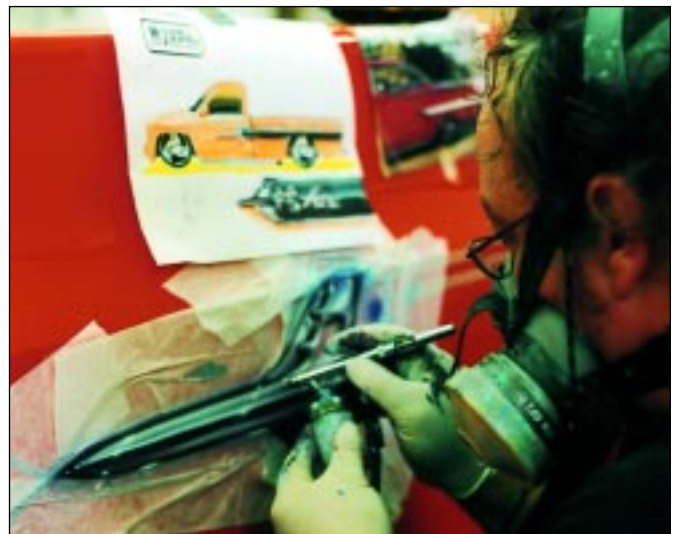
Clean out all of the black and flush the airbrush completely (I use mineral spirits). This last airbrush color is white, so you'll want it to be as pure as possible. And don't over-do the highlights.
