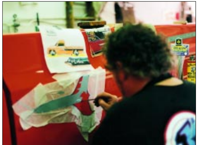
I now mix up 1 Shot imitation silver lettering enamel. (I always add a couple of drops of white for extra body.) Add a drop of "smoothie" fish-eye eliminator to the silver mix. Fill a cup with high-temperature reducer to help the paint flow in hot weather. I don't pre-thin the paint before painting. I prefer to thin only as needed. I now use a #6 brown lettering quill to paint the main portion of the rocket on both sides.
