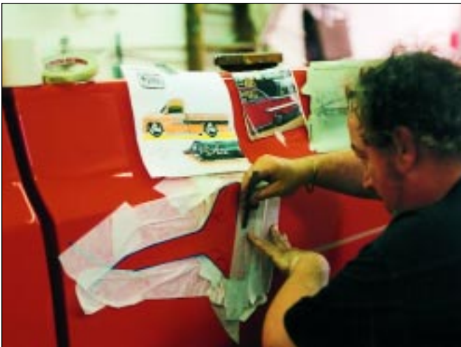
Fine line tape (blue) is used to mask off the rocket. Transfer tape is used to finish off the mask. I cut out the transfer tape using an Olfa knife.
