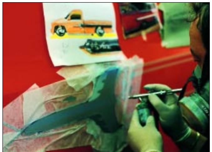
Now the fun begins. I pre-mix all the airbrush colors ahead of time. The paint is thinned at a ratio of 60 percent high-temperature reducer to 40 percent paint. The first color is the lightest of the "sky" colors, 152 blue. I paint across the light silver and the base color. (Note the respirator I'm wearing whenever I airbrush. It has replacement cartridges.)
