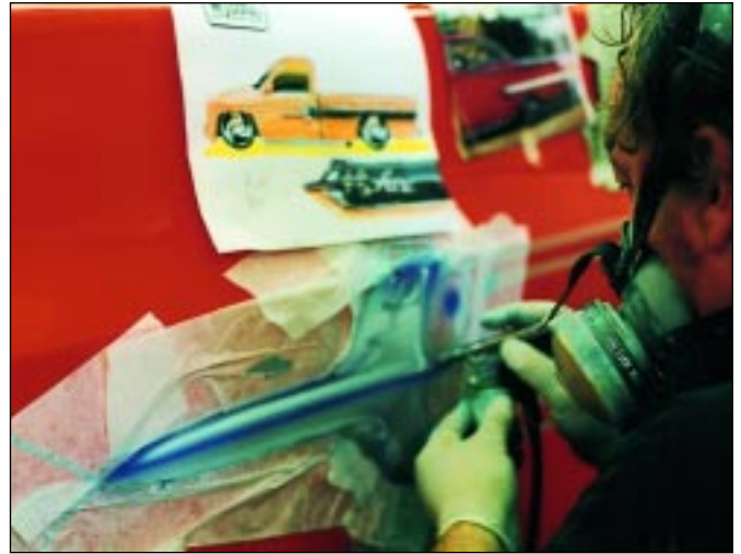
Thoroughly clean out the airbrush. The next color is the white highlight. This is where chrome photos (reference materials) are handy. It's starting to take on a chrome-like look. The bottom also gets some reflected highlights. Keep it simple. Too much white will ruin the effect.
