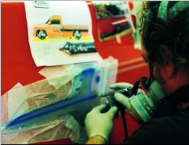
The next color is brilliant blue used to deepen the sky color. This color will go over the light blue in some areas but will not cover it up. Keep this color on the top of the rocket. (Note the disposable latex gloves.)
