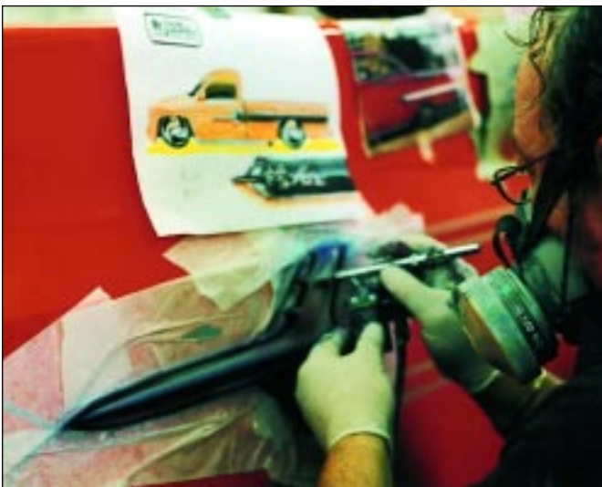
The black is mixed a little thinner than the rest of the colors (I like to make it almost transparent). This allows you to build up the tones a little at a time.
