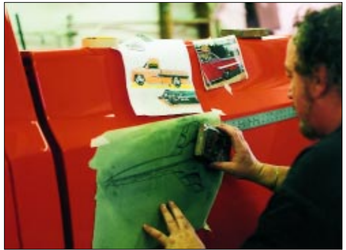
I make a paper pounce pattern of the "rocket" part of the side trim. (Black charcoal powder shows up best.) I lay out the "chrome" side trim using an aluminum ruler with magnetic striping guides glued to the back as my guide. The lines for the trim are drawn with a white Stabilo pencil.
