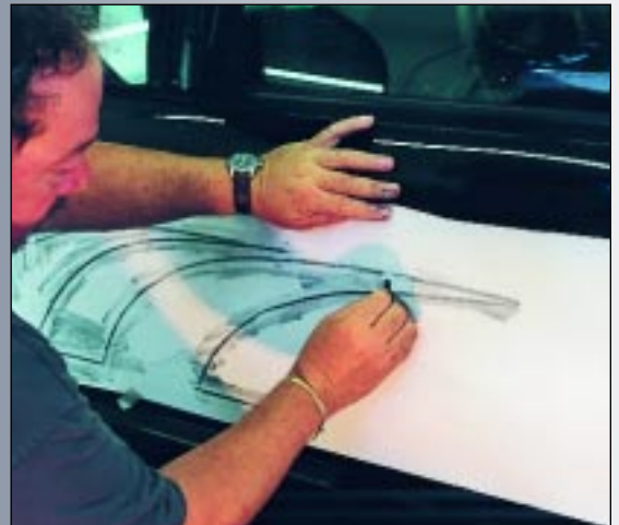
After checking the tape, making sure the straight lines are straight and the curves are smooth, I make a rubbing of the designs. Don't forget, we've got a scratch on the rear fender to hide. I'm using a stick of charcoal, but a graphite stick or a pencil will do just fine. Next I use my Electro pounce to perforate holes in the pattern. I turn the pattern over and using white pounce powder, I transfer the designs to the other side of the truck.
