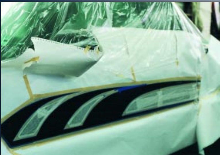
Now comes the hard part, taping up the rest of the truck. I used heavy bond paper (I ran out of the good auto body paper), masking tape and plastic to cover the entire truck. Don't cheap out when masking, buy the best automotive brand you can, and please, please never use newspapers.
