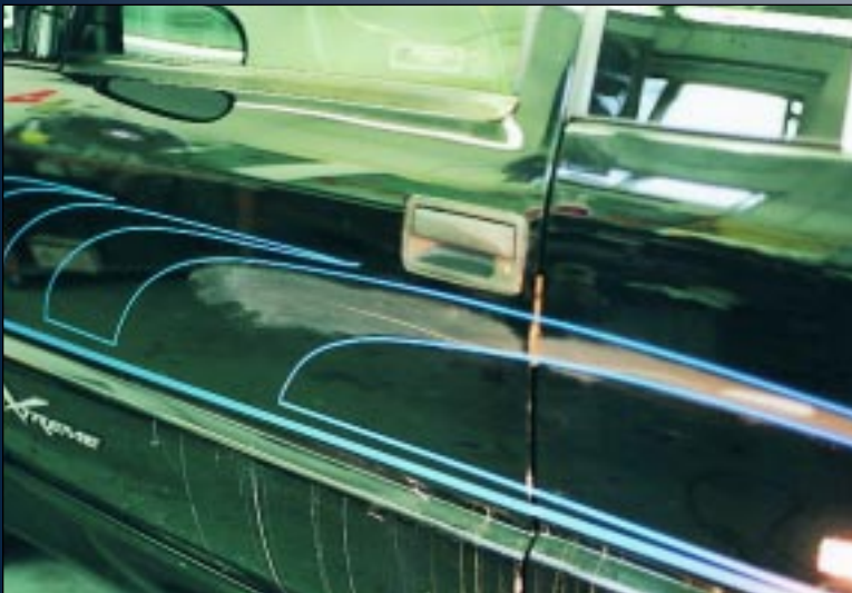
Here you can see that I've already pre-cleaned the sides with Rapid Prep to remove any wax or grease. I've also laid out some blue fine line tape in 1/4" and 1/2" to get a feel for the design. I sand the scratch on the door and cab with 1000 grit wet sandpaper to smooth out the scratch a little. The 1 Shot lettering enamel will fill in what's left.
