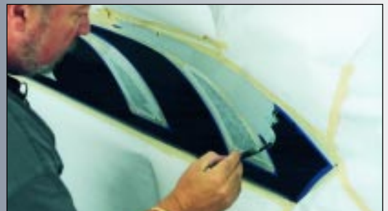
After the designs were scuffed with a 3M Scotchbrite pad, I re-clean the area to be painted with Rapid-Prep (a great water-based wax and grease remover). I'm applying some 1 Shot medium gray lettering enamel (all the paint used on this project is 1 Shot lettering enamel), to which I've added a drop of Smoothie fish-eye eliminator, and a couple of drops of 1 Shot's new hardener for extra strength. I paint this on with a 1" truck-lettering flat. Real "hi-tec", huh? You could also use a sponge roller or a sponge brush.
