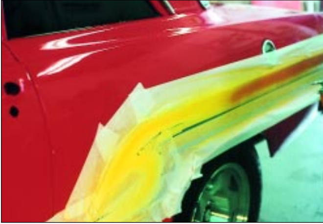
While the yellow tacks up I airbrush medium orange from the rear to just before the design starts to turn down.
