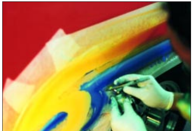
The final airbrush highlights are done with polar white to the top edges of the graphic. Remember, don't get carried away, keep it simple.
