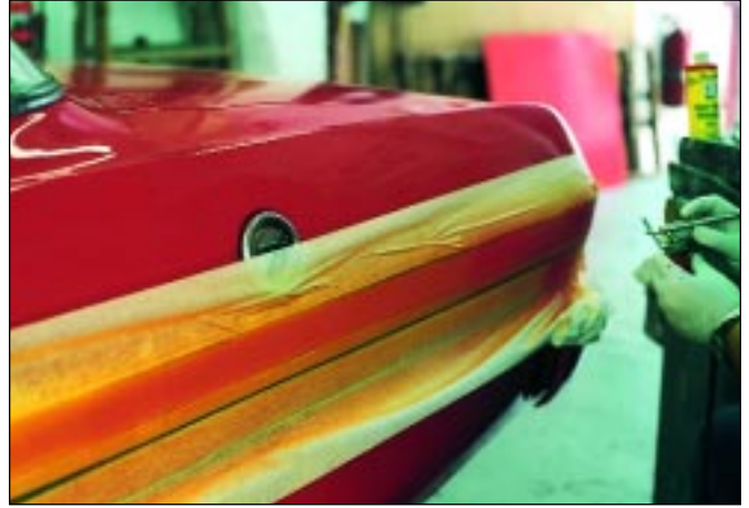
Rubine red is sprayed from the rear to about halfway down the side.
