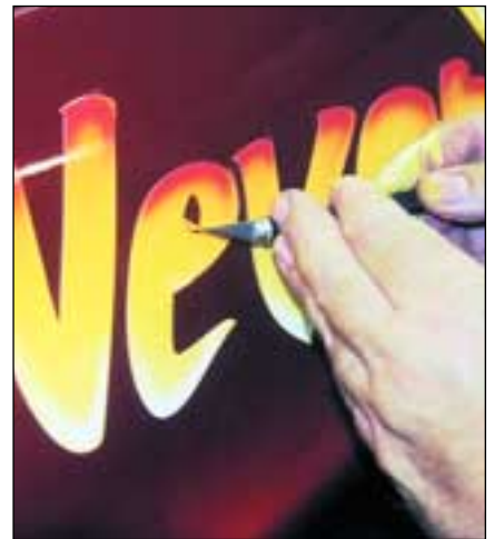
12) This shows you how easy it is to use the paint mask — "no muss-no fuss". I usually wait about 20-25 minutes to remove the paint mask. DO NOT allow the paint to dry completely! If you allow this to happen, the paint will form a "bridge" over the mask and the airbrushing will tear off when you remove the mask.
