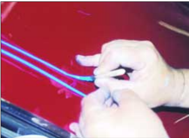
17) I thought I would show you a little pinstriping technique here. Using a "00" Xcaliber striping brush, I add some designs to the side of the roof. I'm using process blue. Note the positions of my hands. The second part of the design connects at the top, and runs parallel with the first part. Check out my pinky, it's like an outrigger used to steady my hand.
