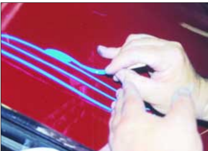
19) Now I fill in a fourth stripe for some weight and add the "tail". If you look close you can see that I used a Stabilo pencil to lay out the stripes. This is a water-based pencil that washes off easily with water and will not affect the paint.
