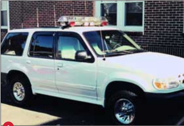
1 This is a brand new Ford Explorer that the town of North Arlington brought to me to have lettered and striped for their Fire Chief. Since I already have the sketch approved, I can start by prepping all the areas that will be lettered and striped. I use Rapid-Tac's Rapid Remover to remove any wax or other contaminants from the truck's surface.
