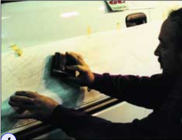
1 I created the layouts in my computer using Vinyl Express LXI 6.6 sign-making software. The file was then pen-plotted and pounced, using the pounce option in my new VE Panther, from Sign Warehouse. Here, I'm, pouncing charcoal powder through the holes in the paper that the plotter made. This will allow me to see the layout that I will paint on the doors.
