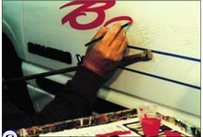
2 I mix 1 Shot bright red (lettering enamel) with some magenta to give it a little more punch. I also add a couple of drops of 1 Shot hardener, for extra strength. High temp reducer is in an Art-Kup, along with the paint. I'm using a No. 6 lettering quill. My trusty Mahl stick helps to steady my hand.
