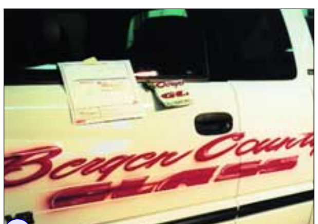
6 I allow the lettering to dry. This can take anywhere from an hour to several hours, depending upon your shop conditions, but the longer you wait the better. Now you can see the overspray that will have to be cleaned off before I can outline the copy.
