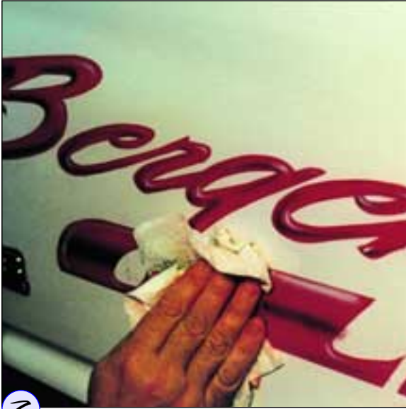
7 I use paper towels moistened with a mixture of mineral spirits and a little water to clean off the overspray.
