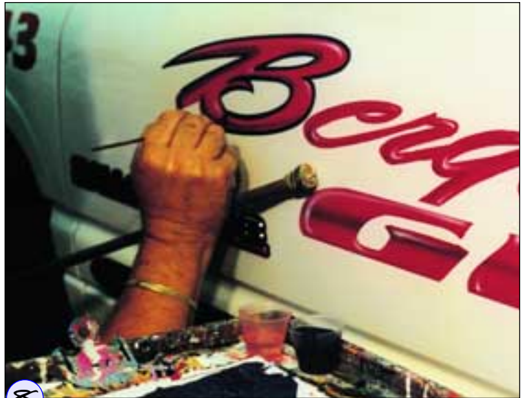
8 A brilliant blue and process blue are mixed for a great covering outline. I use a No. 3 outliner.
