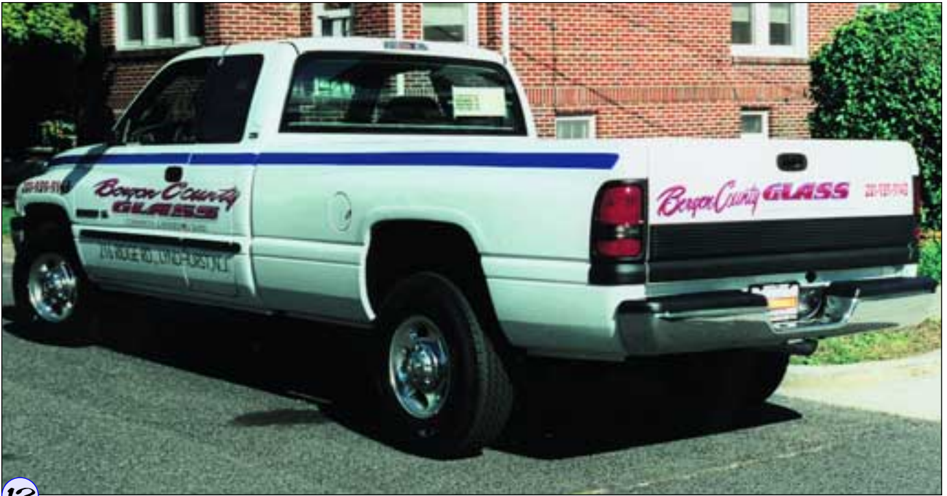
12 The last thing I do is add a 4" Intense Blue stripe down the sides of the pickup, using Oracal's high performance vinyl. I lettered the tailgate to match the doors.
