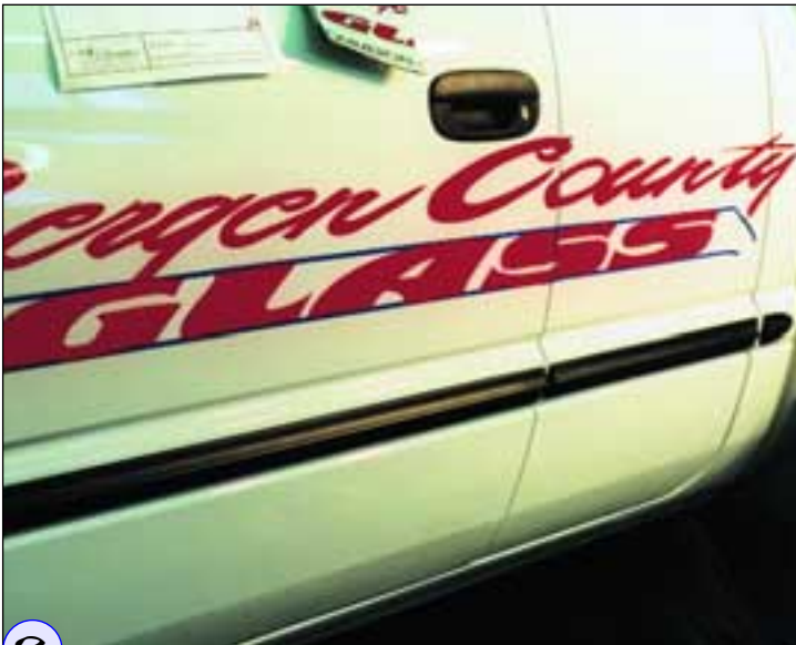
3 After the top line is finished, I move down to the next line of copy. I apply some blue fine line tape, on top and bottom. I use the same lettering brush for this copy.
