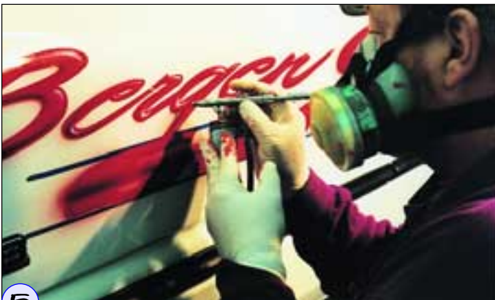
5 Here I'm using 1 Shot white on the opposite side of the script, to create highlights and give the script a rounded look. Also you can see that I'm wearing a charcoal respirator.
